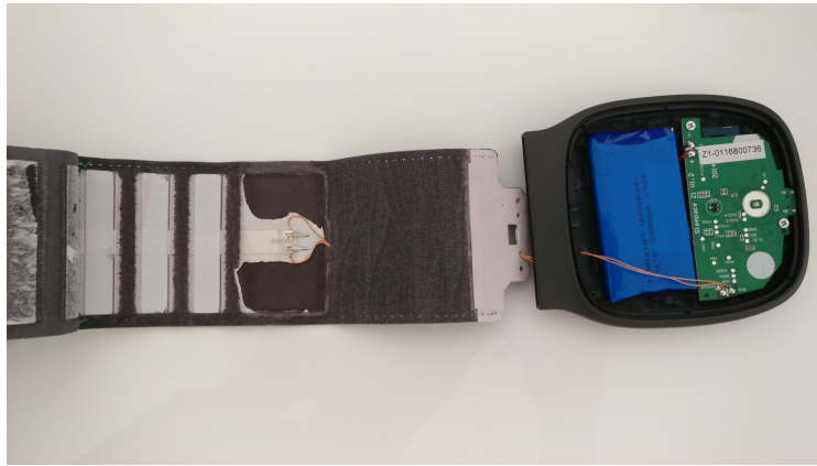
Figure A.1: Removing the foam material reveals two wires inside the SleepAce.
